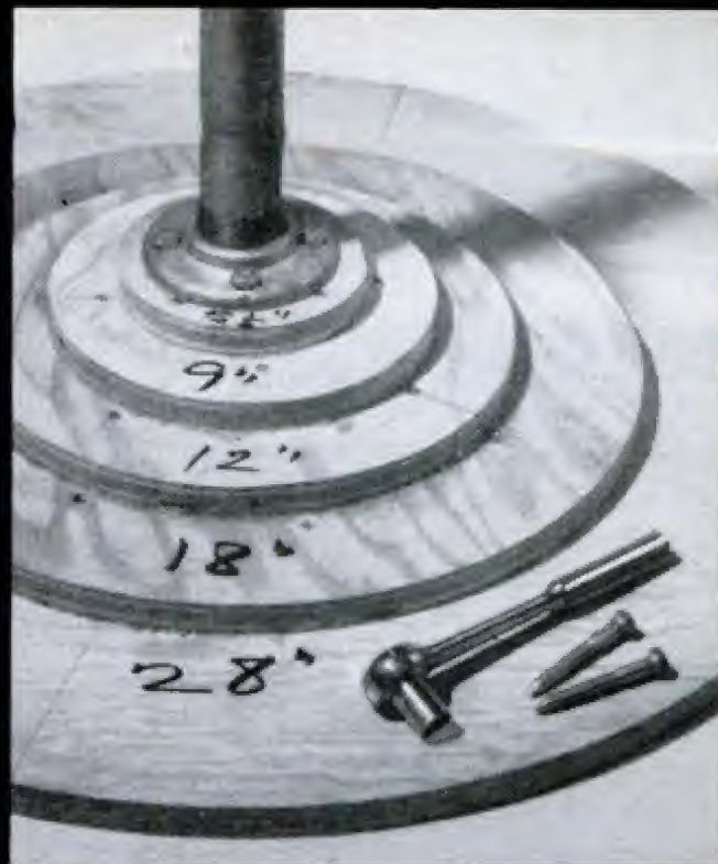
PEDESTAL BASE is formed of glued-together, concentric plywood discs. Pipe determines table height
